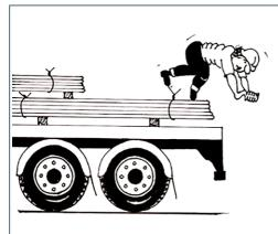
**DO NOT** climb up the fabric on the vehicle. Use a ladder or another appropriate means of access, such as a gantry platform. If a ladder is used, ensure that it is secured.
